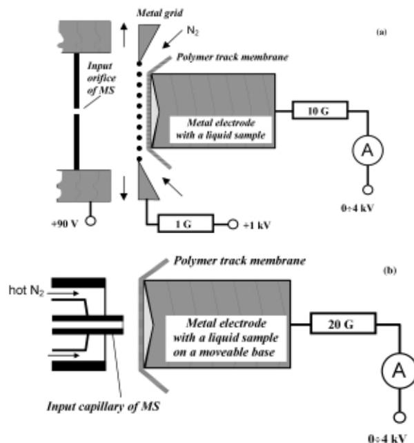
**Figure 1.** Set-up diagrams of the atmospheric-pressure membrane-based liquid-sample ion source employed with: (a) ToF mass spectrometer; (b) FT ICR mass spectrometer.
