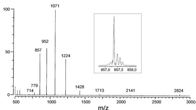
**Figure 6.** Bovine ubiquitin AP-EMI FTICR mass spectrum. Note that the space-charge effect reduced the resolving power.
