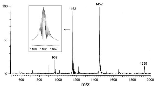
**Figure 5.** Human insulin AP-EMI FTICR mass spectrum. Note that the space-charge effect reduced the resolving power.
